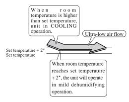
In Heating operation, after start the unit, the air conditioner will sending warm air a moment later to prevent the cold air blowing out. In Dehumidifying, when the room temperature drops 2\* higher than the set temperature, regardless the set fan speed, the air conditioner will intermittently operate in low fan speed.
